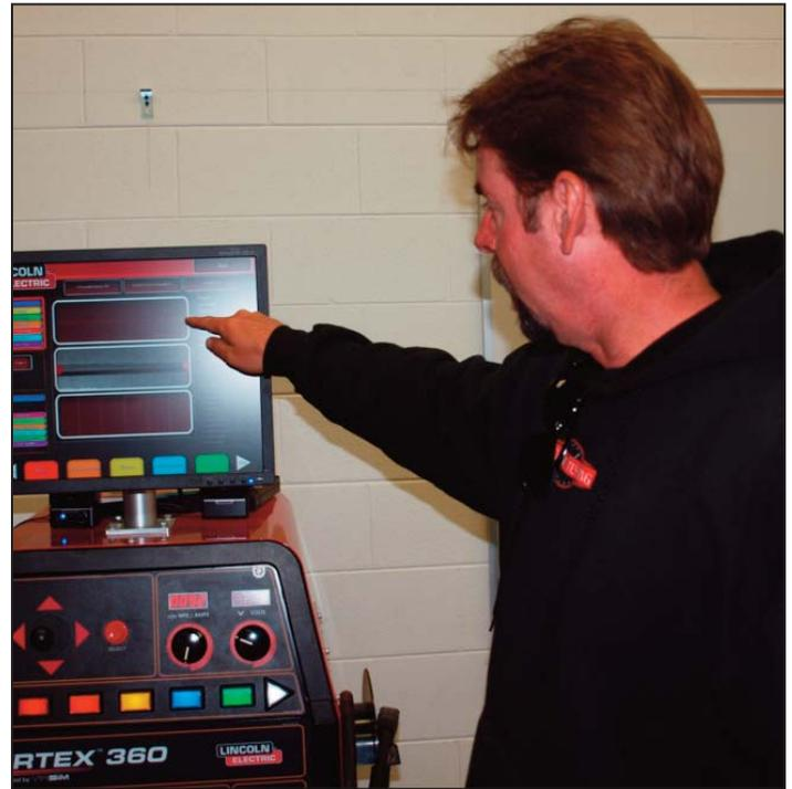
LCC welding instructor Doug Cash (pictured above) works with students Dustin White (top left) and Michael Bolser (bottom left) demonstrating the welding simulator. The simulator is used to teach the fundamentals of the program without the cost of welding supplies. The machine allows the students to simulate a weld like they were on an actual job site.
